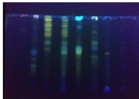
Figure 2. TLC fingerprint of “ Monzej-e-balgham ” and the corresponding ingredients. Stationary phase: silica gel; Mobile phase: ethyl acetate: formic acid: glacial acetic acid: water (100:11:11:26); Reagent: natural product; The fingerprint from left to right corresponds to Adiantum capillus veneris , Glycyrrhiza glabra , Rosa damascena , “ Monzej-e-balgham ”, Onopordum acanthium , Pimpinella anisum , Ficus carica and Vitis venifera .
