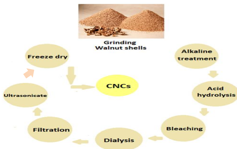
Figure 1. Graphical presentation of the cellulose nanocrystals synthesis steps
