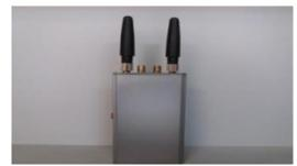
Figure 1. Electromagnetic field-producing device (2100 MHZ).
