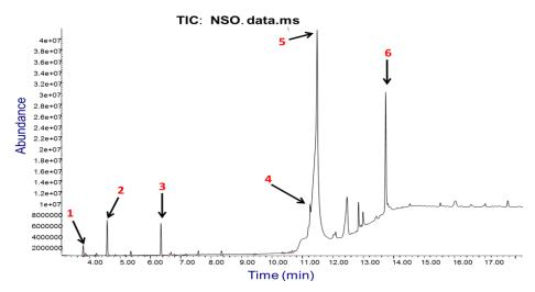
Figure 1. GC-MS chromatogram of *Nigella sativa* seed oil. Major peaks identified are: (1)  $\beta$ -thujene (RT=3.802 min); (2) o-Cymene (RT=4.590); (3) Thymoquinone (RT=6.357); (4) Oleic acid (RT=11.260); (5) Trans-13-octadecenoic acid (RT=11.488) and (6) E, Z-1, 3, 12, nonadecatriene-5,14-diol (RT=13.741).
