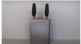
Figure 1. Electromagnetic field-producing device (2100 MHZ).
