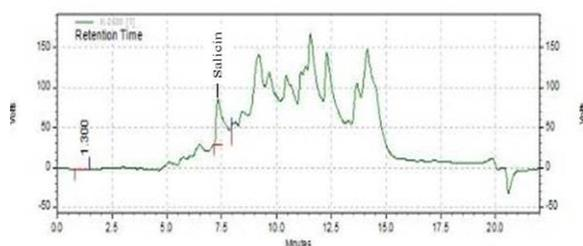
Figure 1. RP-HPLC chromatogram of *salix alba* extract. Chromolith Performance Nucleosi (250 × 4.6 mm; C18 5 µm) column – mobile phase: water/methanol, v = 1.2 mL/min, UV detection at λ =265 nm
